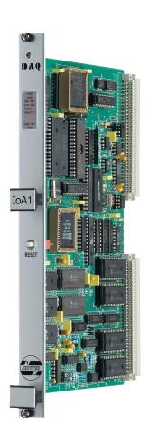
Offering reliable, high-speed operation, the Callisto IoA1 module collects analog data and performs a wide range of power system calculations.
